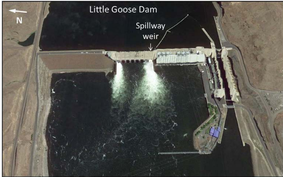
Figure 1.4. Aerial photograph of Little Goose Dam. The spillway weir (surface route) is located on the south side of the spillway.
