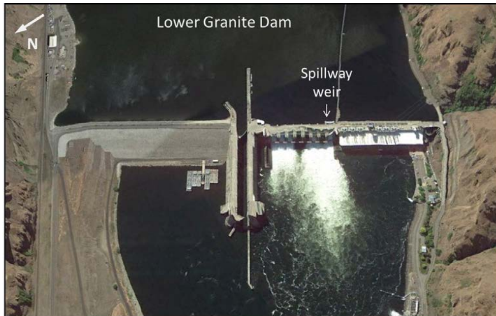
Figure 1.3. Aerial photograph of Lower Granite Dam. The spillway weir (surface route) is located on the south side of the spillway.
